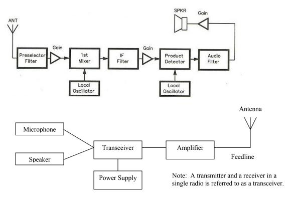
Block Diagram for a Typical Amateur Radio Station
